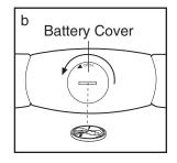
Remove the old battery from the sensor unit. Insert a new **CR 2032 battery**, making sure that the writing is on top. In addition, make sure that the rubber gasket is in place in the sensor unit. Replace the battery cover and turn it to the closed position.
